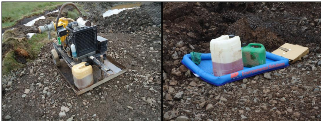
Plate 12: examples of drip trays and bunds
